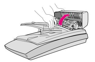
2 Lift the large green tab (located to the left of the roller) and gently remove the jammed page.
